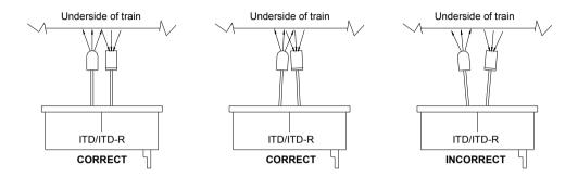
It is recommended that the ITD-R is mounted under your layout and the IR sensor pushed up between the sleepers in the centre of your track. Drill two 4.0mm (5/32 inch) holes with 5mm between their centres or make a 4.0mm x 9.0mm slot, being careful not to damage the track. Screw the IR sensor in place, adding a spacer if necessary so that the top of the IR sensor sits level with the top of your ballast or sleepers.
